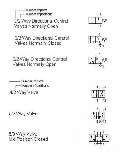
Figure 3.2 Symbolic Representation of Directional Control Valve
