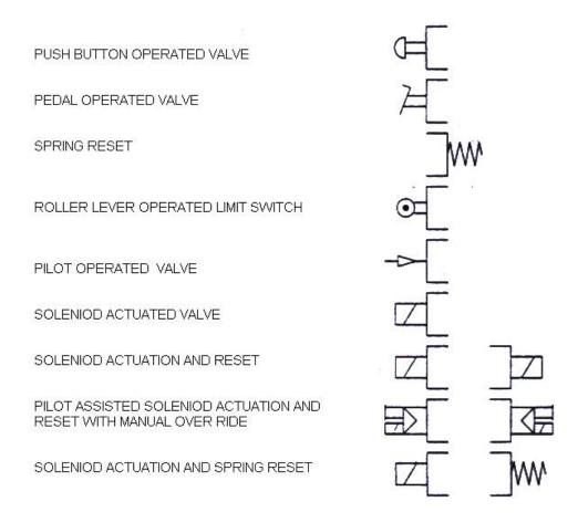
Figure 3.3 Method of Actuation and Reset of Directional Control Valves
